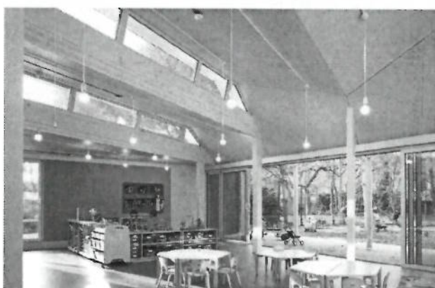
Figure 2-8 Clerestory windows are effective at adding natural light to activity rooms.
