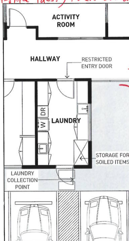
Figure 2-17 A typical child care facility laundry layout. External access may be provided if laundry is done off site or for deliveries.
